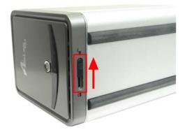
Step 2 Slide the front panel up and then pull it off to access the drive bays.
